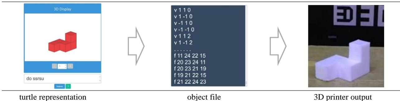
**Figure 2. 3D printing process using 3D turtle representation system**
