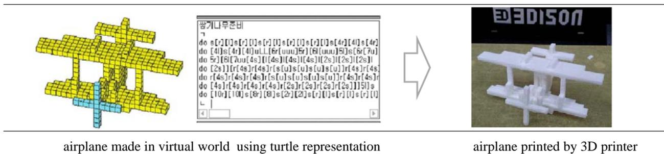
**Figure 4. Airplane made in both virtual and real world**
